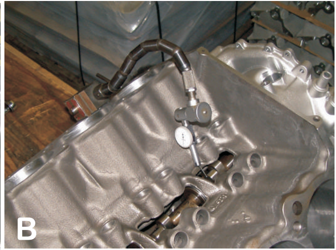
B. Dial indicator set up to measure end play
