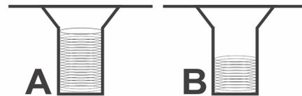
6. For best results we recommend running a bottoming tap through each bolt position. This will ensure that each bolt torques properly.
